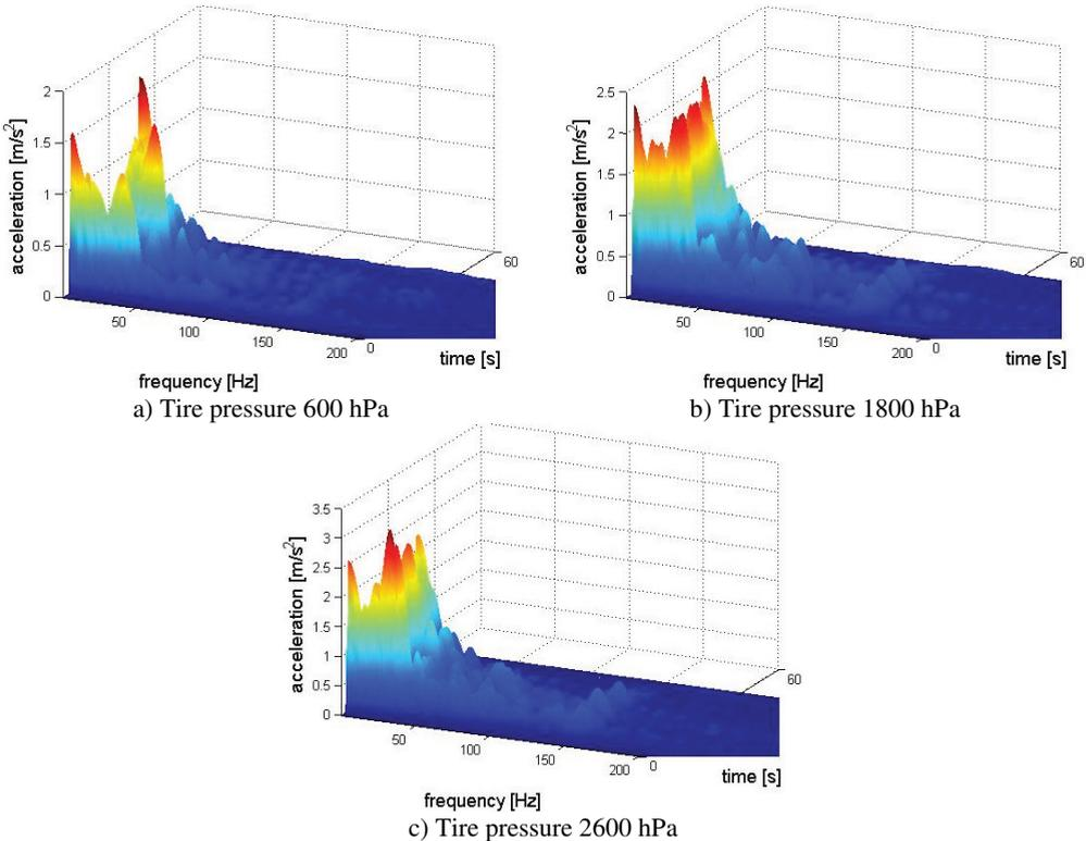
**Fig. 8.9.** Time-frequency distribution of the vibration of floor under driver's feet
