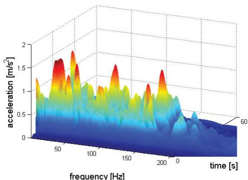
a) Shock absorber with 100 % of liquid volume
