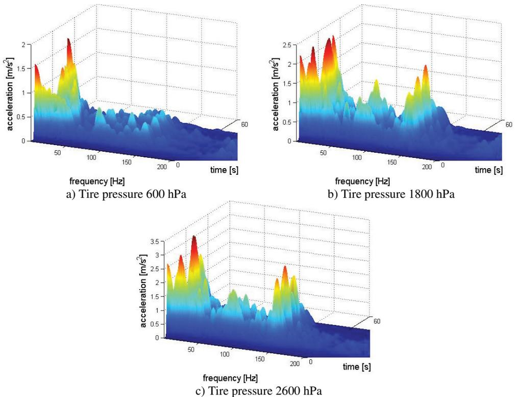
**Fig. 8.11.** Time-frequency distribution of the vibration of floor under rear left passenger's feet
