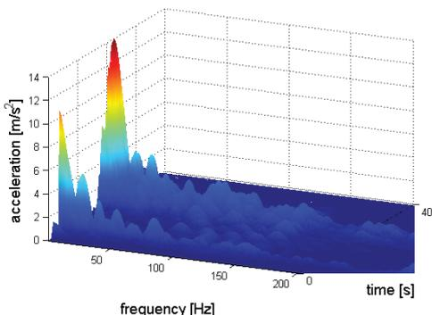
b) Shock absorber with 50 % of liquid volume
