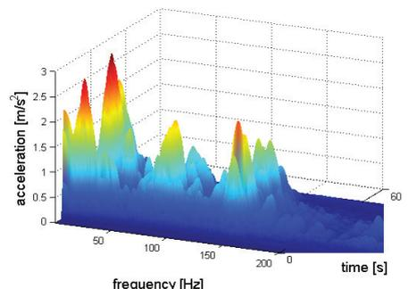
a) Shock absorber with 100 % of liquid volume
