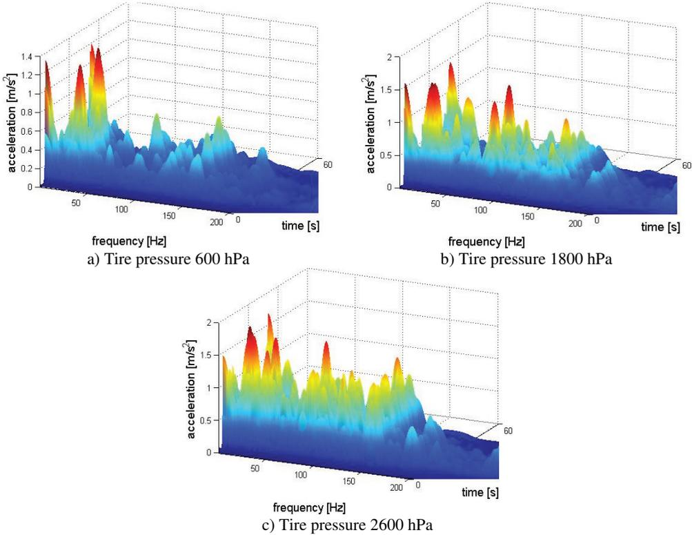
**Fig. 8.12.** Time-frequency distribution of the vibration of floor under rear right passenger's feet
