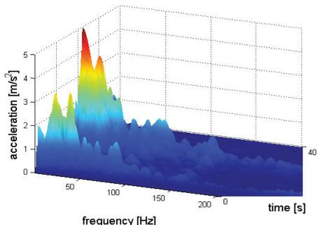
b) Shock absorber with 50 % of liquid volume
