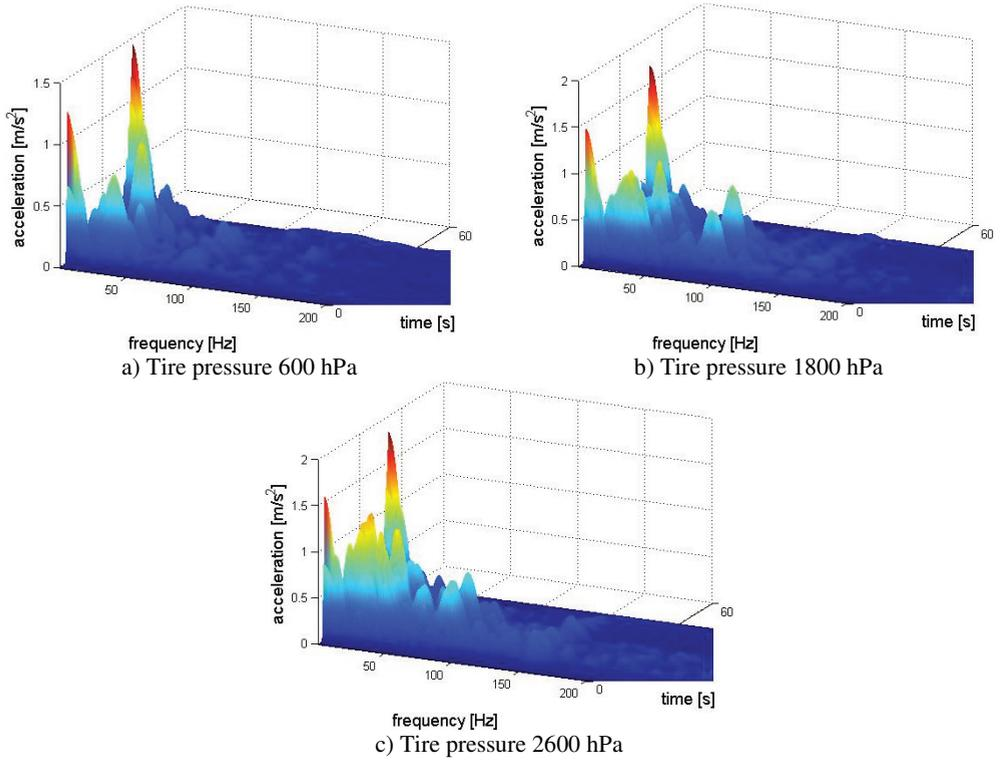
**Fig. 8.10.** Time-frequency distribution of the vibration of floor under front passenger's feet
