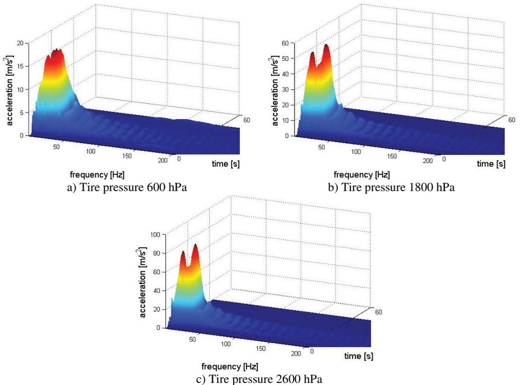
**Fig. 8.7.** Time-frequency distribution of the vibration of suspension arm
