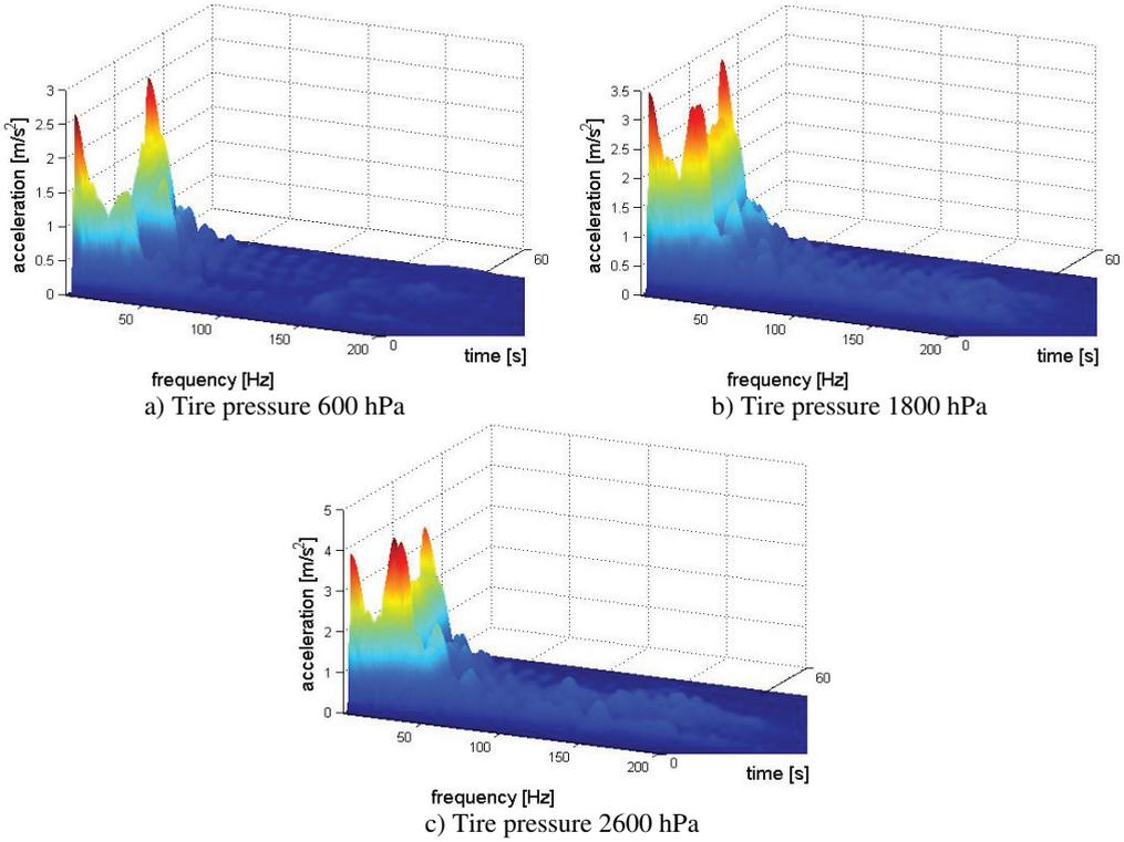
**Fig. 8.8.** Time-frequency distribution of the vibration of upper mounting of shock absorber
